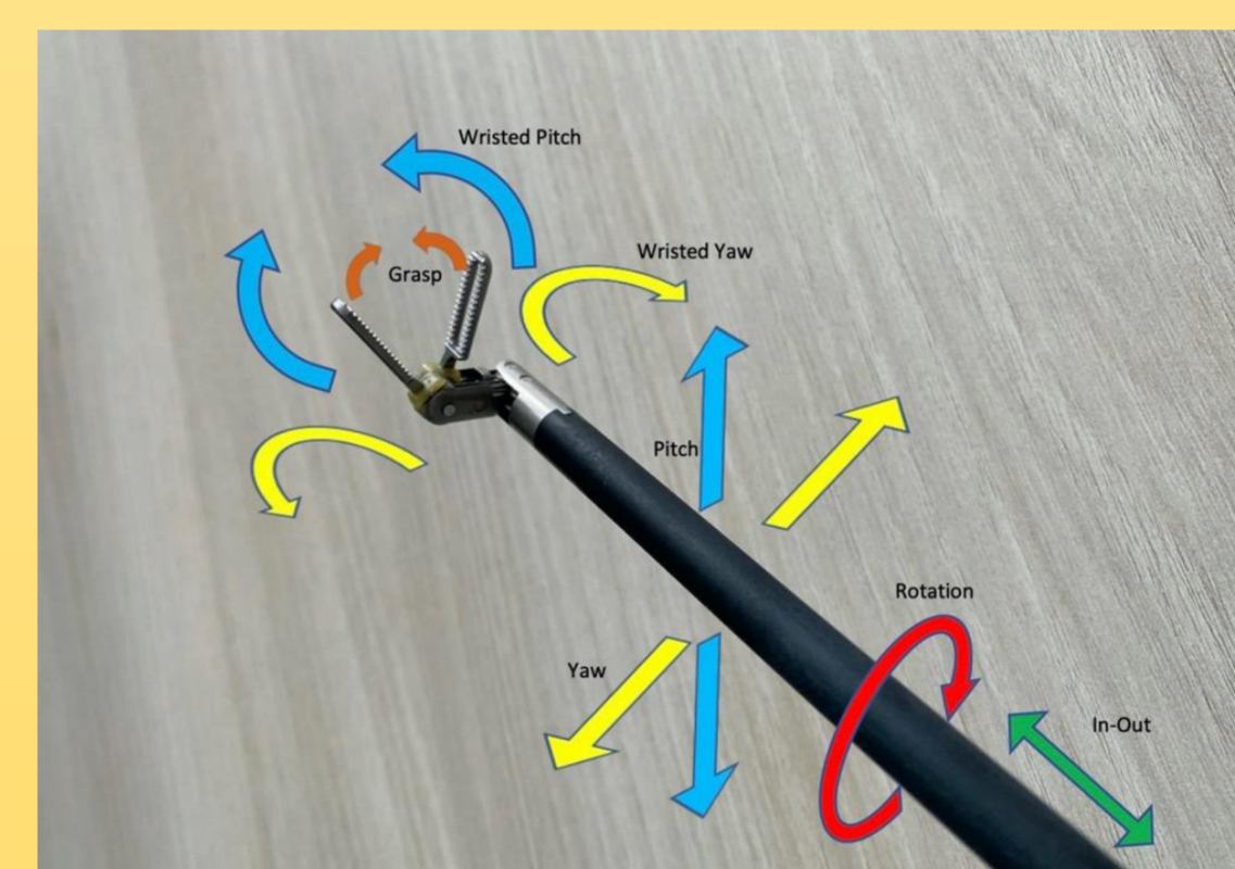
Fig. 3: The range of motion of the Artisential® end effector.
